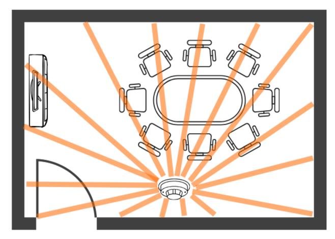
In settings where the view of a sensor might be blocked by obstacles like cubicle walls, using dual technology sensors or adding extra PIR sensors can help maintain a clear line of sight. Dual technology sensors are recommended for areas with limited movement, such as private offices, open offices, restrooms with stalls, and libraries. However, they are not ideal for places with continuous movement, such as hallways and warehouses.
