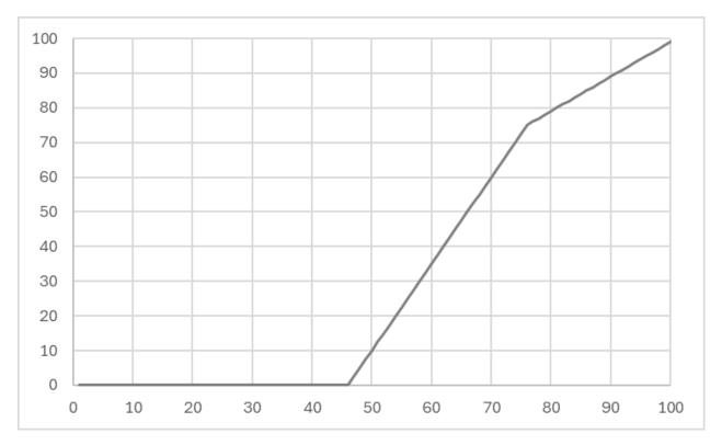
In this example, the Lamp\_2\_Offset is set to 45, and the Lamp\_2\_Limit is set to 75.
