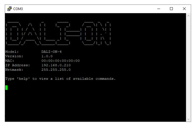
The command-line interface is accessible with serial console software such as PuTTY on a computer.
